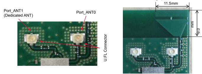
The 50ohm microstrip line and Type2EL\_Antenna needs to be copied when module is installed in the End product.
