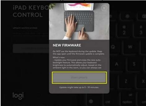
NOTE: Remember to keep the keyboard attached, the app open, and refrain from using the keyboard or touchpad during the process.
