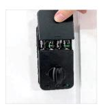
Remove the battery cover, install AAA1.5v batteries, and close the battery cover.
