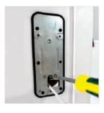
Align the holes of the built-in board and fix them with flat head screws
