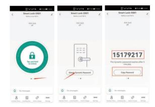
Swipe left on interface 1; enter interface 2; click "Get dynamic password" on interface 2; generate a dynamic password; enter the password to unlock the smart lock.
