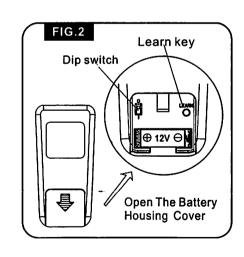
● Note: Install the 12-volt battery (not included) to the remote control.
