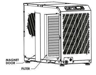
**Step 6.** Remove sticker near drain line and ensure the vent hole is unrestricted.
