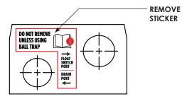
**Step 7.** Install drain line. No need for p trap or knot in drain line. Drain downward at >3 degree. Ensure PVC drain is pitched downward.
