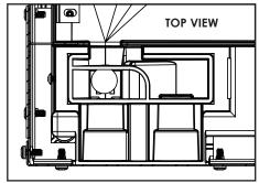
Step 4. Replace cover back and install torque screw.
