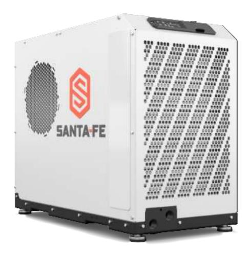
The **Santa Fe Advance Dry110** is designed for superior dehumidification in basements, crawl spaces, and attics. It features industry exclusive dual exhaust outlets for maximum space drying and installation flexibility. Other features included an onboard digital control with a terminal block, dew point cut out, and a low maintenance built in P-trap.
