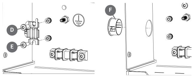
**Step 5**. Route wires through 7/8" hole and secure using the clamps intended for conduit or cable. There is a hardwire jumper kit included with the unit.
