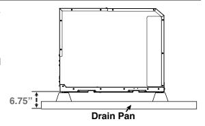
The unit features an industry exclusive dedicated float switch port (float switch is not provided and must be purchased separately) to shut the Advance Dry110 off in the event the main drain port clogs or fails. In order to use this feature, the internal plug needs to be knocked out. If the unit is located above or in the living space, according to code, a secondary drain pan is to be placed under the unit and a float switch should be wired to the dehumidifier.
