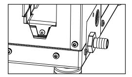
Step 5. Reinstall filter and magnetic door on unit.
