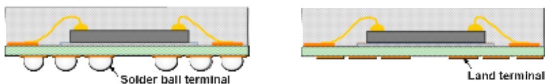
Figure 4, Definition of BGA and LGA
