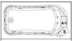
Standard (S) & Alternate (A-1) Pump Locations Pump must be located at A-1 position when ordered w/ a heater
