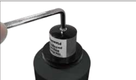
1 Loosen the fork mounting screws. Take the gaskets out.
