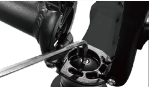
2 Put the handlebar into the fork and lock the screws.
