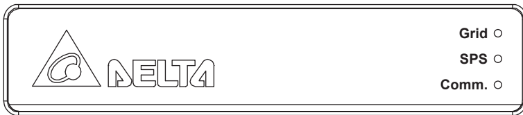
Figure 2-7 : LED indicators of DELTA BX6.3_AC
