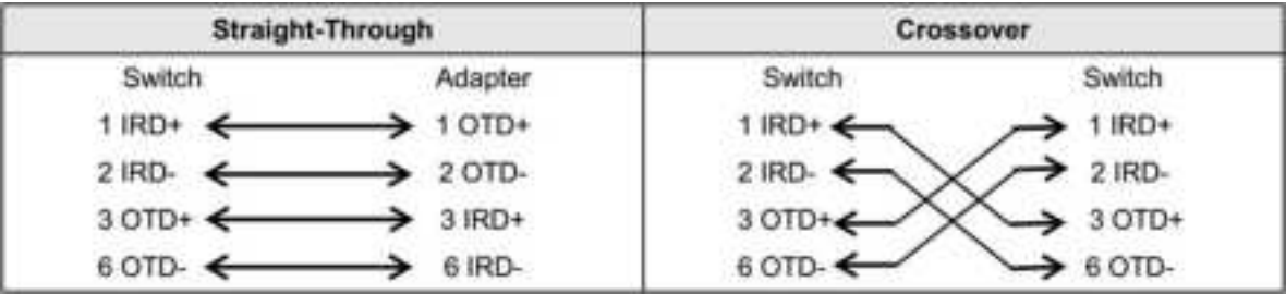
Figure 6-3 100BASE-TX/10BASE-T Twisted Pair Connections
