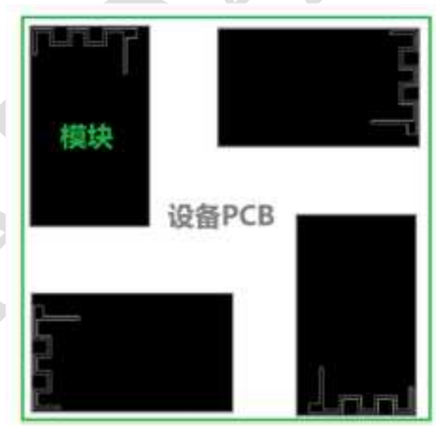
Fig 11-2 Recommended PCB layout
