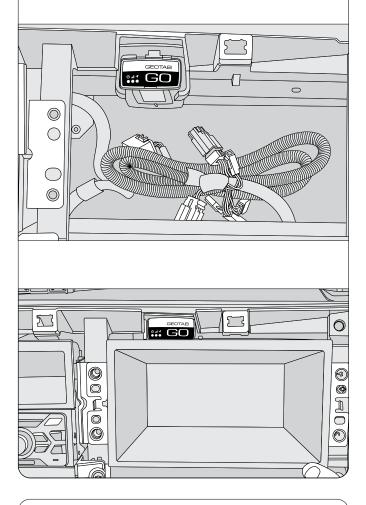
**Step 4 :** Complete an install check for the GO device. Once the install check is done, reinstall all dash panels.
