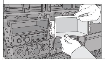
**Step 1:** Remove the dash panel, and then remove the two panels/compartment holders to the right of the radio.
