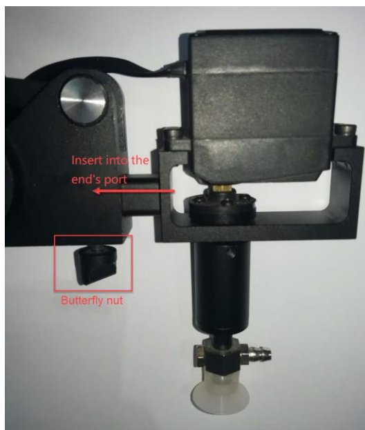
Figure 5.8 Install a suction cup kit
