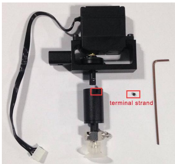
Figure 5.12 Dismantle the suction cup
