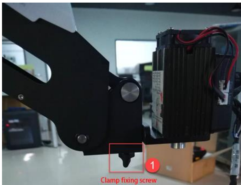
Figure 5.60 Fasten the laser with clamp fixing screw
