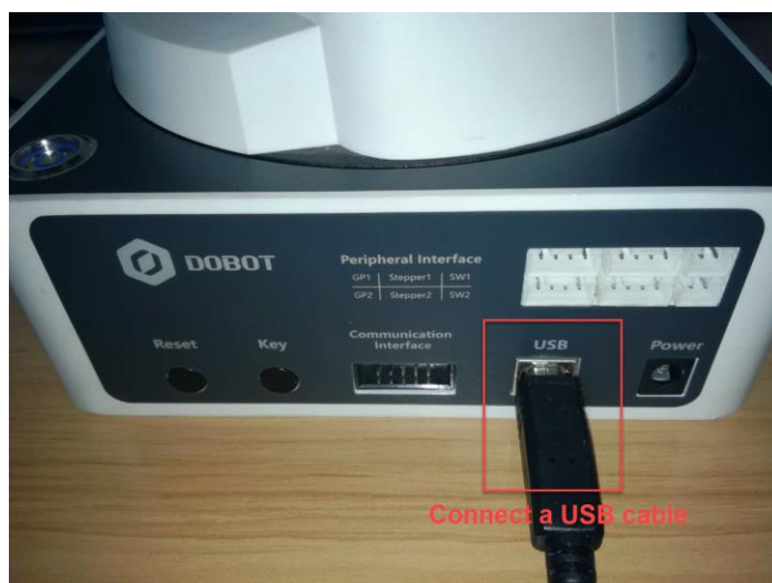
Figure 2.2 Connect the Dobot Magician to your computer
