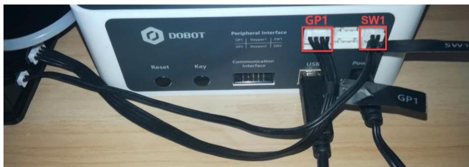
Figure 5.7 Connect the air pump to the Dobot Magician
