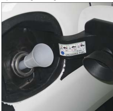
Emergency Fuel Filling Procedure
