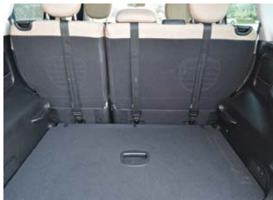
Rear Seat Tether Strap Mounting
