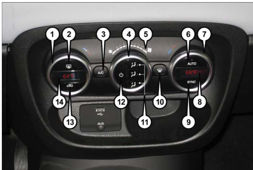
Automatic Temperature Controls (ATC)
