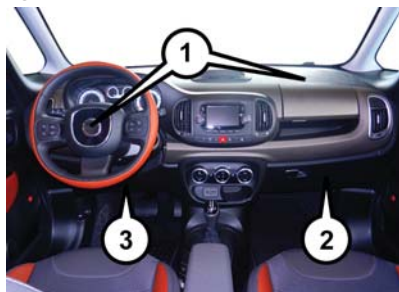
Front Air Bag/Knee Impact Bolster Locations
