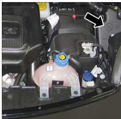
Front Distribution Unit
