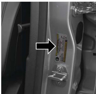
Example Tire Placard Location (B-Pillar)
