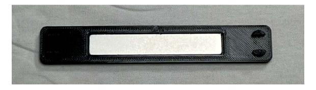
After the magnet is placed into the mount, it can now be installed onto the chassis. Take your index finger and place it over the middle of the magnet and place your thumb over the middle of the flat side of the mount. Now pinch the parts together (this is to ensure that the magnet will not fall out during the installation process).
