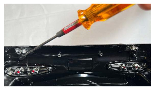
Install the rear body mount using the original screws from the taillight assembly and the middle portion of the rear bumper. Use the remaining screws to fasten the posts that have the spacers installed. A picture of the installed rear body mount and spacers can be seen in the picture below.
