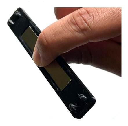
While holding the mount and the magnet together, take one side of the mount and align the clips with the hole which was previously used for the rear body posts. Remember to keep the marked portion of the mount facing towards the rear. With your free hand, apply equal pressure on the flat side of the mount opposite to where the clips are located until there is a click which indicates that the mount was seated properly. When installing the clips into the chassis it's recommended to go slow.
