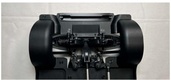
Now place the washers onto the screws and drive them into the front chassis mount. Do not tighten them all the way just yet. Perform one last check to see if the mount matches the pictures seen above. If they do not match the pictures above then adjust them and tighten the screws. DO NOT OVER TIGHTEN!!! This can cause the part to strip and jeopardize the holding strength of the mount.
