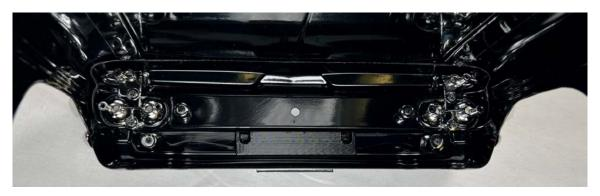
Take a 60x10x3mm magnet and place it onto the front chassis mount. Make a note on what side the magnet is attracted to the front chassis mount (again it is recommended to mark this side with a permanent marker).
