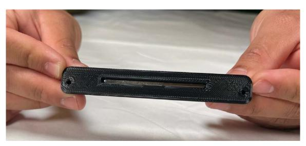
After the magnet is properly seated, the mount can be installed onto the chassis. Start by locating the M3x8mm screws and the washers from the kit. This hardware will be used to secure the front chassis mount using the existing holes from the stock front body posts. Next examine the shape of the front chassis mount. It should be noted that on one side there is a flat surface which needs to be facing the front of the chassis when the mount is installed. With this in mind
