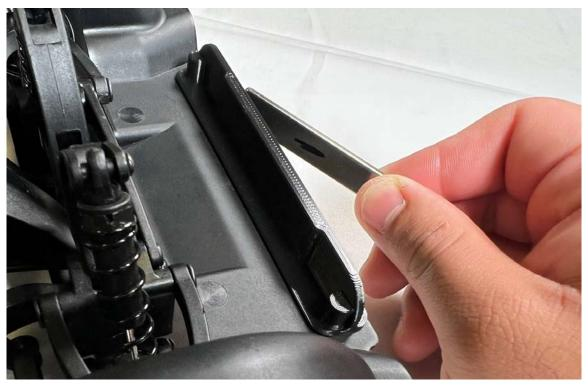
Insert the marked magnet into the empty slot of the mount having the marked side facing away from the front bumper. It's best to start with the corner of the magnet pressing against the tab and sliding it until the tab overcomes the magnet as seen in the pictures below.
