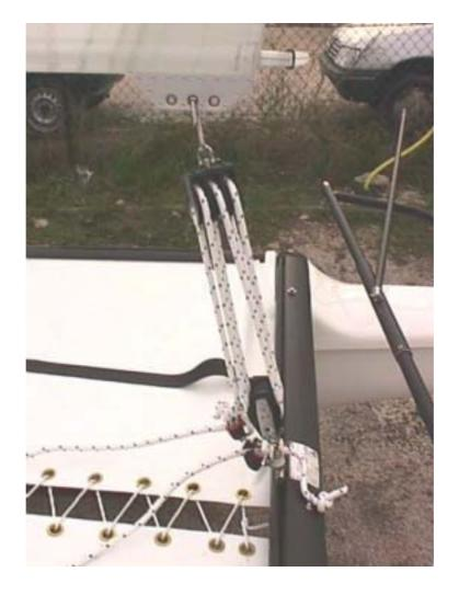
Tie the cunningham line to the grommet in the sail tack using a bowline knot or similar. Pass the line down around the cunningham cleat and back through the grommet. Pull down on the line, apply sufficient tension to remove wrinkles from the sail luff and cleat off at cunningham cleat.
