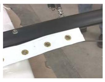
ldentify the right and left side trampoline halves and insert them into the trampoline track in the back of the rear crossbar. Pull them all the way to the deck edge.
