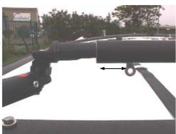
Assemble the stay adjusters with twist toggles, clevis pins and split rings. Attach them to the anchor bar pins. Ensure that the stay adjuster points fore and aft - as per photograph.
