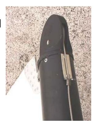
When the sail is all the way to the top of the mast, engage the slug on the halyard wire into the halyard lock. Secure the halyard line to the cleat on the side of the mast. Stow the excess line in one of the trampoline pockets.
