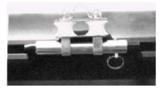
Reassemble the traveller car in a reverse manner, i.e.: fit in the upper part, slide the cylinder and place the pin and the split ring.
