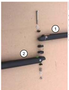
Attach the tiller crossbar (1) to the tiller arm (2). Pay attention to the left and right side. Insert the screw as shown on the drawing. Repeat the same operation on the other side.
