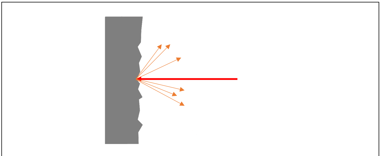
Figure 3 Reflection of the laser beam at the surface of an object
