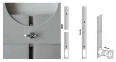
**Step 4:** Close your window to secure the kit in place. It needs to hold the windows kit firmly in place, secure the window kit with duct tape if required. It is recommended that the gap between the adapter and the sides of the window should be sealed off for maximum efficiency.
