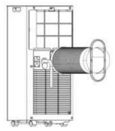
**Step 6:** Adjusting the length of the flexible exhaust hose, to make sure the distance between the unit and the window will be more than 27.56 inches, height from exhaust hose to the floor will be more than 35.43 inches. And avoid bends in the hose. Then place AC near an electrical outlet.
