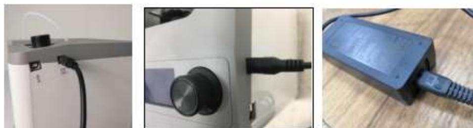
Flip the power switch on the AC power adapter to the ON position (I). After the printer finishes booting, you will see the following wizard. Depress the Knob on top of the printer to select Next on the Welcome screen, then again to select Next on the STEP1: LOAD FILAMENT screen.
