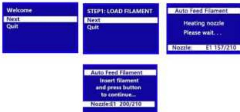
Using a pair of scissors or side cutters, cut about an inch off the end of the filament, then gently straighten the end of the filament. Squeeze the lever on the Extruder, Insert the filament into the bottom until you encounter resistance, then release the lever.
