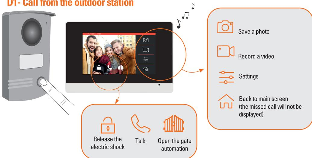
The diagram shows an outdoor station on the left and a monitor on the right. The monitor displays a video call with a family. A red circle highlights the call control icons on the right side of the video: a camera icon, a video camera icon, a settings icon, and a home icon. An arrow points from this circle to a grey rounded rectangle containing the following options:
