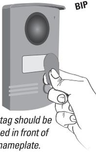
The tag should be placed in front of the nameplate.
