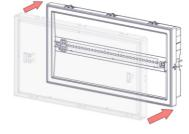
Attention!! The 6 plastic latches (A) must be secured (click sound). This requirement is important to ensure the IP65 rating. Power on the luminary.
