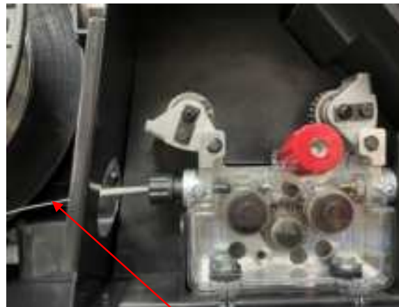
(4) Snip the wire carefully, be sure to hold the wire to prevent the spool uncoiling. Carefully feed the wire into the inlet guide tube of the wire feed unit.
