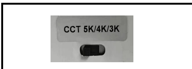
CCT Dip Switch (3000K/4000K/5000K)
