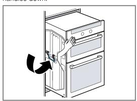
**4.** Push the appliance in fully. Do not kink or trap the connection cable, or route it over sharp edges.
