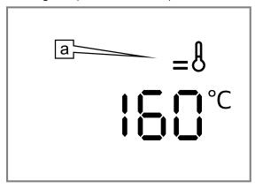
When you are preheating the appliance, the optimal time to place your food in the cooking compartment is when the & symbol first goes out.
