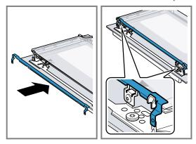
**12.**Attach the door cover ① and use a screw to secure it on the left- and right-hand sides ②.
