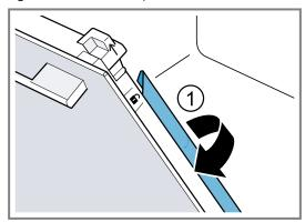
8. Pull the first and second intermediate panels upwards and out at an angle, and set them down carefully on a flat surface.
