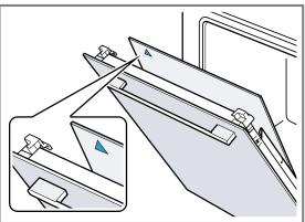
1. Slide the first intermediate panel into the lowest retainer ① and fit it at the top.
