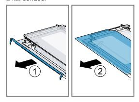
9. Loosen the screw on the left- and right-hand spacers a 1 and remove both spacers 2.
