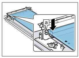
7. Place the two spacers a on the left- and right-hand sides onto the arrow of the upper intermediate glass pane.
