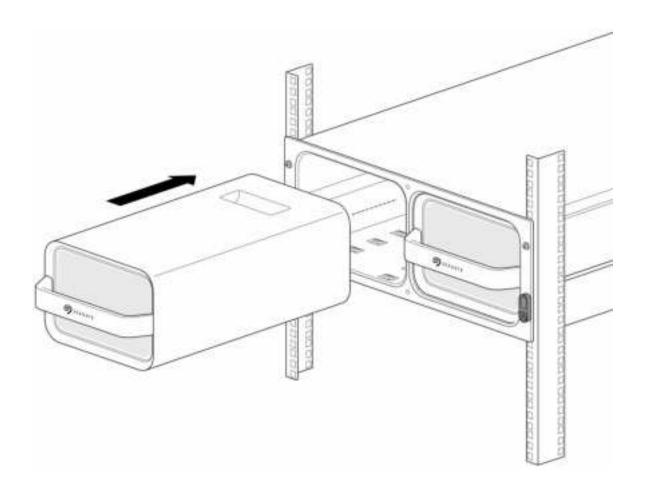
Slide device in until it's fully inserted and firmly connected to Rackmount Receiver's data and power.
