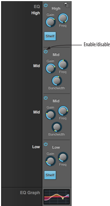
Figure 8-3: The Four-band parametric EQ module.
