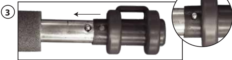
5 Align the opening on the pole cap with the spring-loaded button on the top of the Upper Poles. Then, slide the Pole Caps (Q) over all 8 Upper Pole assemblies until the buttons click into place.
