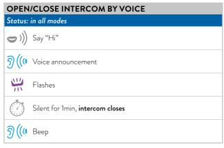
**Note:** the voice activation is possible only with an intercom paired to the **Control button-Rider 1 (VOX must be active)**
