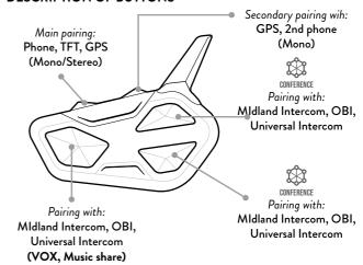
To carry out any pairing, you need to access Settings. If the Control button is pressed less than 7 seconds, the device will turn on instead of accessing Settings. Should this happen, repeat the procedure.
