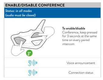
**Note:** in Conference mode, the deviced paired with Vol+/Vol- are temporarily dosconnected.
