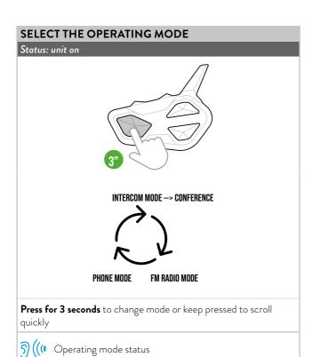
**Note:** By pressing briefly **Vol** + and **Vol** - together, BTR1 Advanced communicates the selected operating mode.
