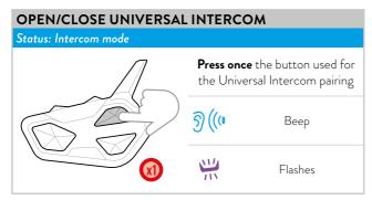
**Note:** to open/close the audio from a **different brand device**, use the voice call command (for some models it is necessary to send the voice call twice)
