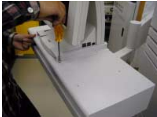
19. Attach the two attachment by four screws (0515-2079) and washers (3050-0893) to fix the FPD.
