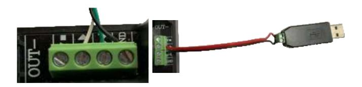
Once the cables have been connected to the voltage converter unit in accordance with the instructions in the image and table, connect the device to the PC via USB. in the Device Manager under "Ports (COM & LPT)", check which port the voltage converter unit is connected to; in this example it would be COM4.
