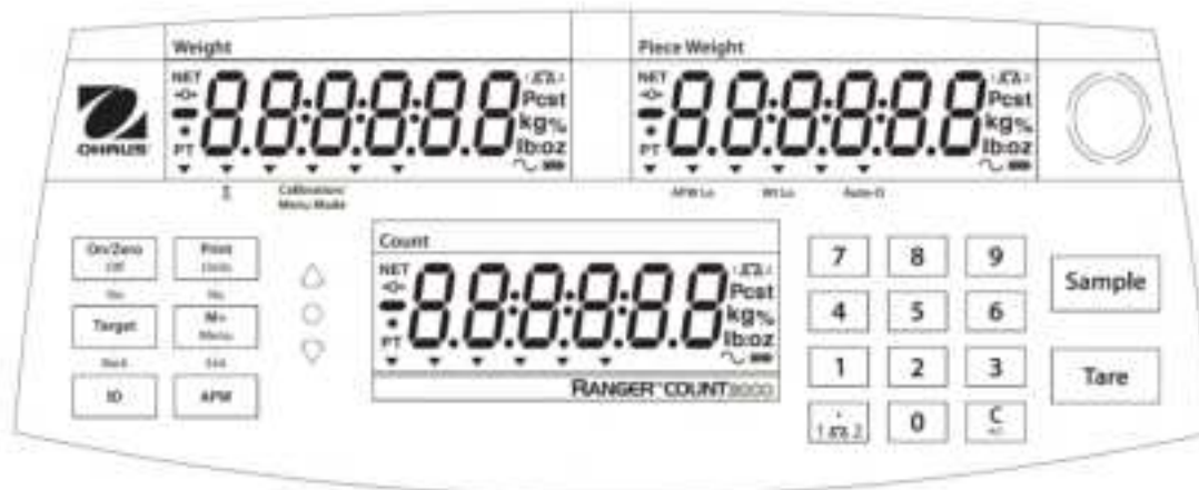
Figure 3-1. Ranger Count 3000 Control panel with LCD displays
