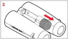
Next, pull the central focusing unit's wheel up slightly (Figure 2).
