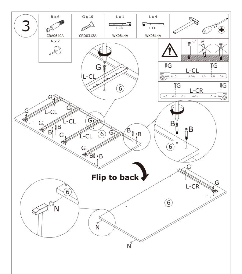
As shown in the figure, screw the self-tapping rod (B) into Panel 6. Use the screw (G) to fix the sliding rails L (L-CL) and L (L-CR) to Panel 6.
