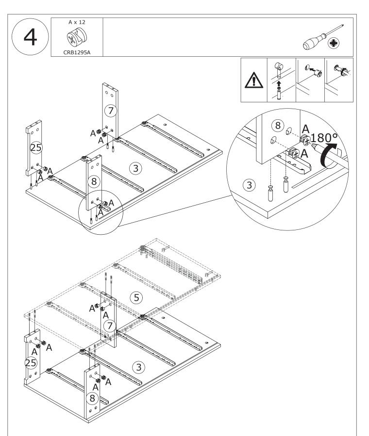
As shown in the figure, connect Panels 7, 8 and 25 to Panels 3 and 5, and then insert the eccentric wheel (A) and tighten it by rotating it clockwise.
