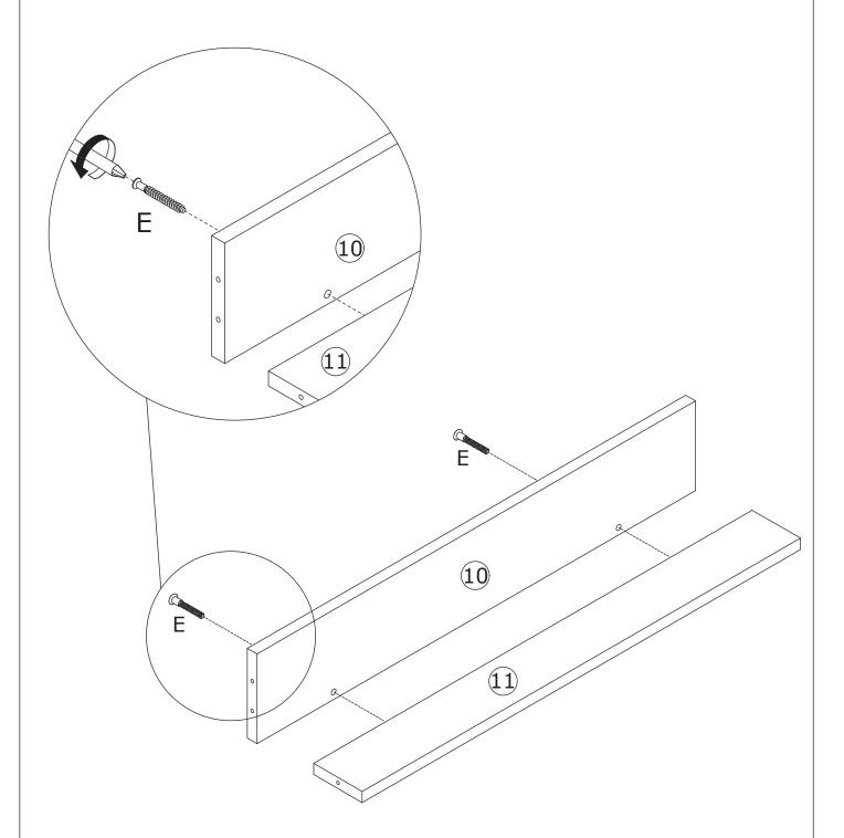
As shown in the figure, use the screw (E) to fix Panel 10 and Panel 11.
