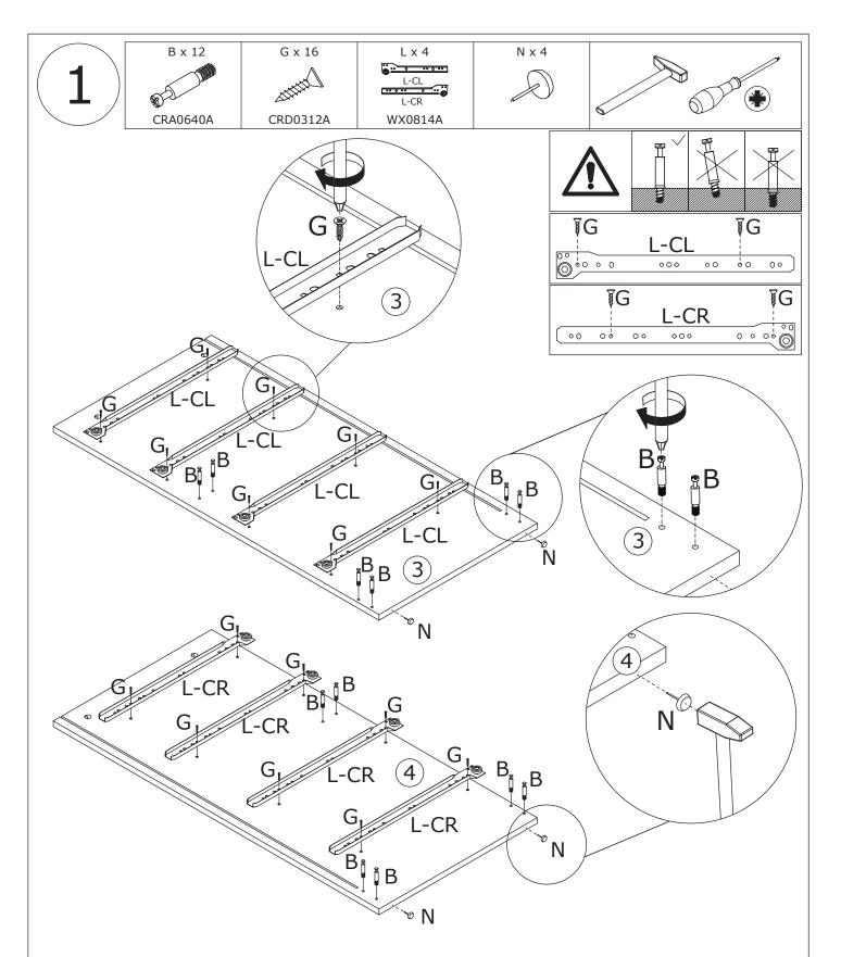
As shown in the figure, screw the self-tapping rod (B) into Panels 3 and 4.
