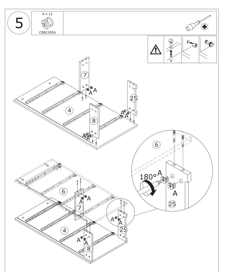
As shown in the figure, connect Panels 7, 8 and 25 to Panels 4 and 6, and then insert the eccentric wheel (A) and tighten it by rotating it clockwise.
