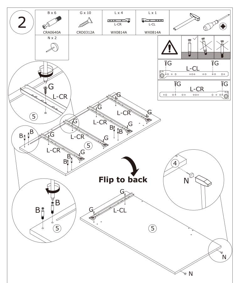
As shown in the figure, screw the self-tapping rod (B) into Panel 5. Use the screw (G) to fix the sliding rails L (L-CL) and L (L-CR) to Panel 5.
