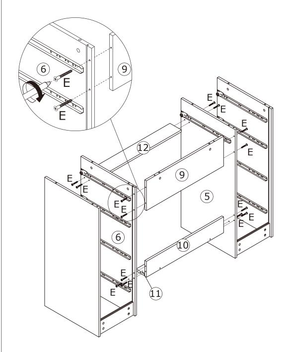
As shown in the figure, use the screw (E) to fix Panels 9, 10 and 12 to the assembled unit.
