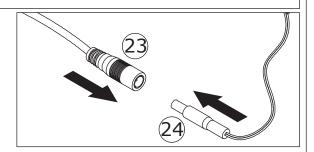
As shown in the figure, connect Wires 23 and 24.
