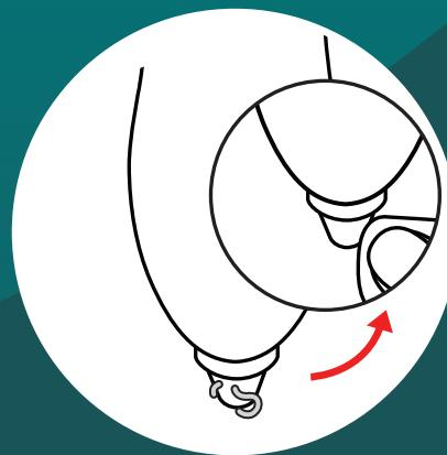
If you have trouble extruding, try cleaning away any plastic that may be stuck to the nozzle while the pen is switched on.
