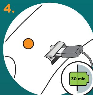
When your 3Doodler Start+ is fully charged, the LED light will stop flashing and change to SOLID ORANGE.
