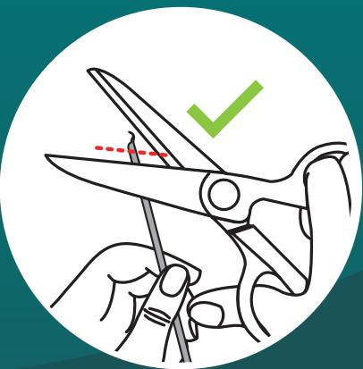
Snip the tip of a partially-used plastic strand before re-inserting into the pen.
