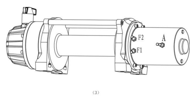
After the remote control and the main unit of the electric control box are assembled. The connection between the electric control box and the winch: Connect to the outlet of the electric control box according to the F1, F2, and A positions corresponding to the winch motor in the picture above.
