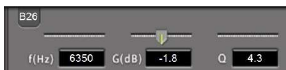
Example of IIR pole adjustment
