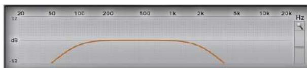
Crossover frequency 80 - 2000 Hz @ 12 dB/Oct.
