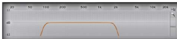
Crossover frequency 80 - 2000 Hz @ 48dB/Oct.
