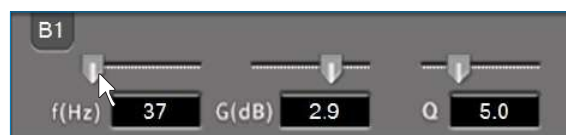
Example of IIR pole adjustment
