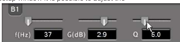
Example of IIR pole adjustment
