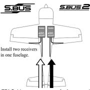
**FDLS-1** is a secure system. In the event of trouble with the main receiver, the **FDLS-1** will automatically switch to the sub receiver and fly safely.
