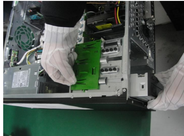
Figure 12 Remove the PSU from Cage
