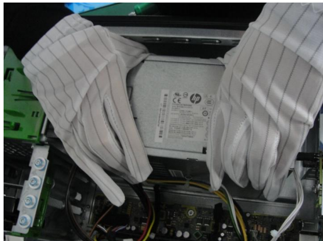
Figure 12 Remove the PSU from Cage
