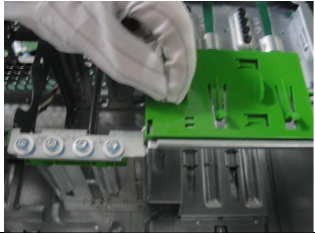
Figure 28 Remove cable clip from chassis
