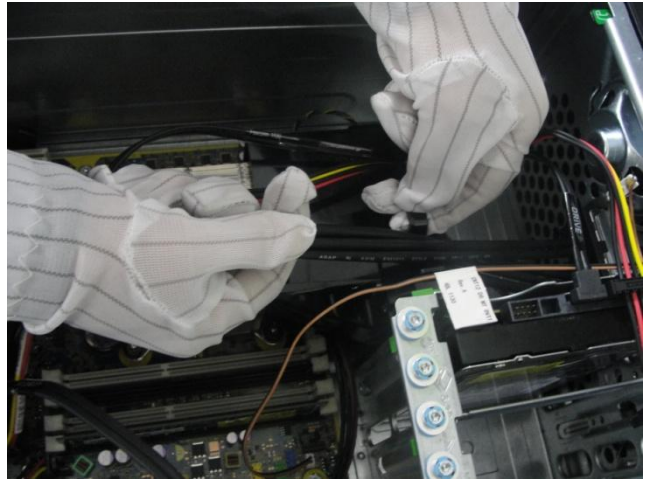
Figure 4 Remove front system fan from the chassis
