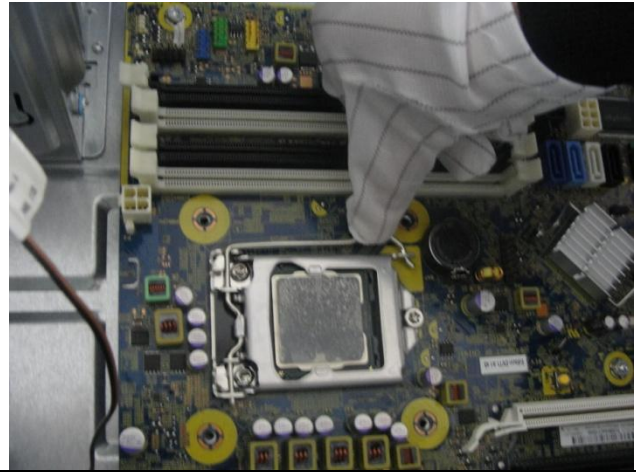
Figure 22 Remove the battery from the system board
