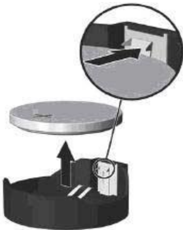
Figure 23 Remove the battery from the system board
