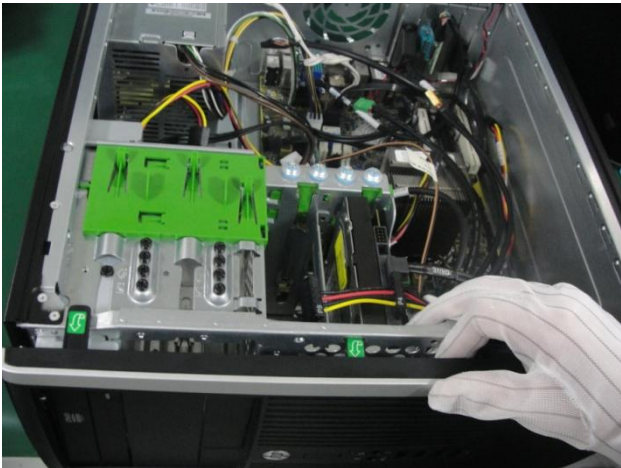
Figure 11 Loose the PSU's screw from chassis
