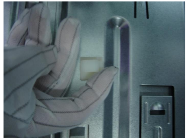
Figure 30 Remove the system fan from fan duct
