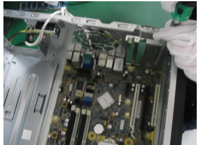
Figure 24 Loose the screws of MB from chassis
