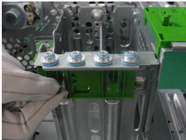
Figure 29 Loose the screws of fan from the fan duct
