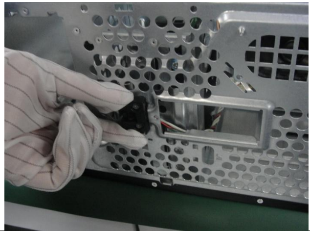
Figure 18 Remove the Memory card from the board
