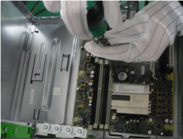
Figure 21 Remove the CPU from the board
