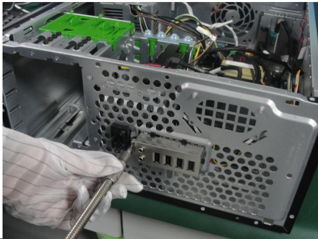
Figure 17 Loose the screws of speaker and remove it
