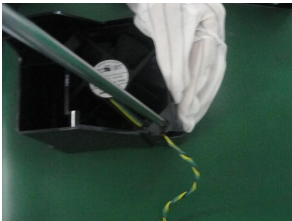
Figure 29 Loose the screws of fan from the fan duct
