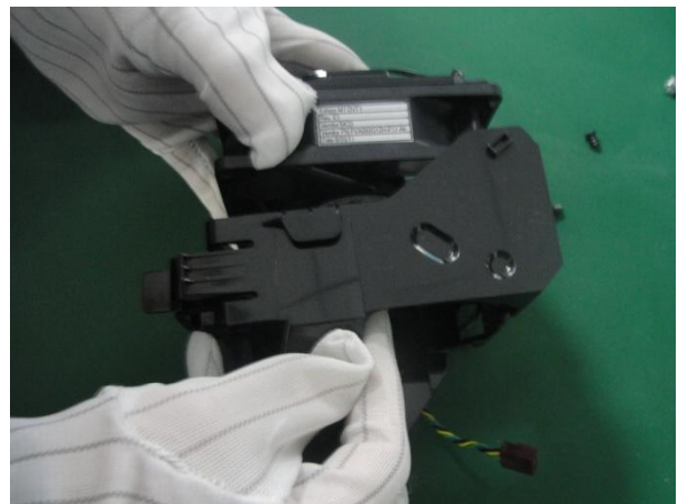
Figure 30 Remove the system fan from fan duct
