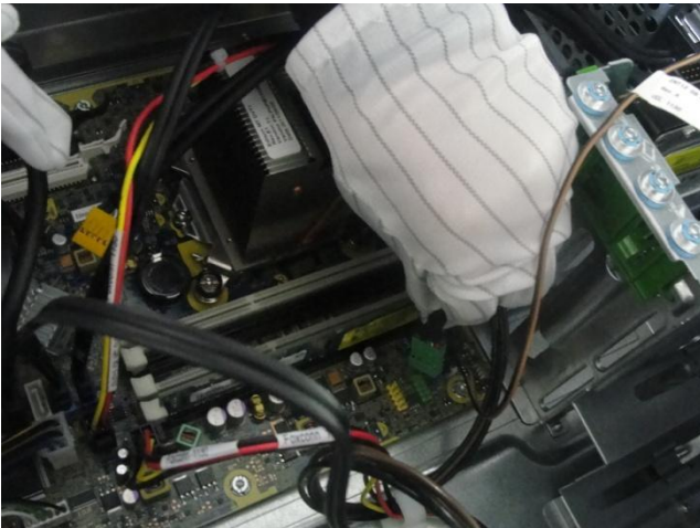
Figure 5 Disconnect CPU Power cable from the MB
