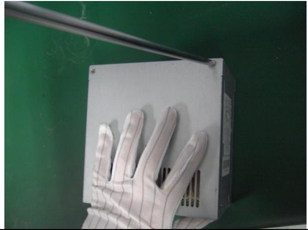
Figure 34 Remove the four screws on the board
