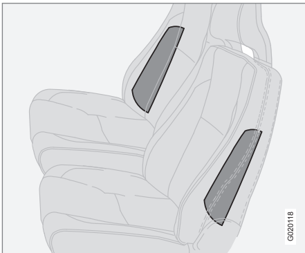
Location of the side impact (SIPS) airbag
