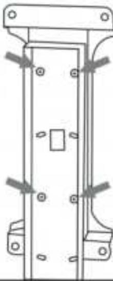
2. Place the support wallboard to be installed, mark the hole position and punch holes, put the expansion pipe into the hole, and fix the support body through the wallboard with the expansion screw.
