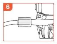
Connect one end of outlet hose pipe with the oulet end of the machine.
