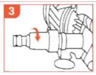
Screw the inlet filter clockwise to attach with the main unit.
