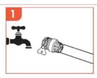
Attach one end of the inlet pipe with the tap connector
