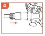
Push and attach the inlet connector with the inlet filter.
