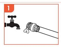
Attach one end of the inlet pipe with the tap connector
