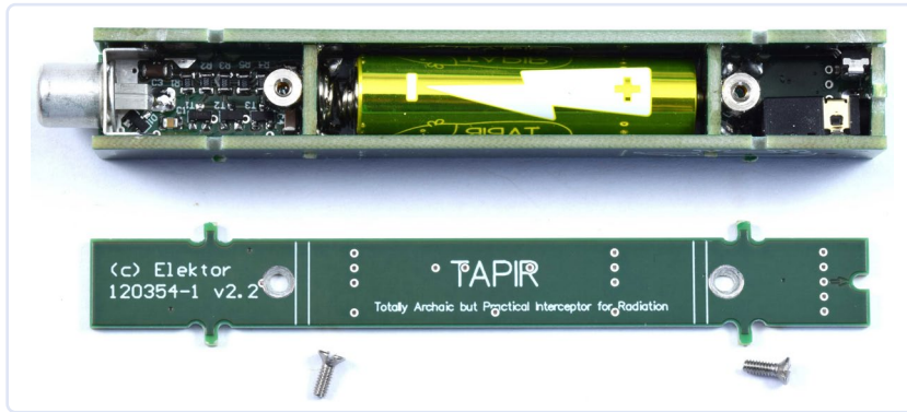
Figure 22. The AAA battery inserted. Notice polarity!
