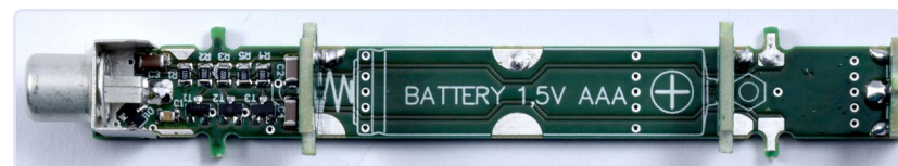
Figure 16. PCB 3 with PCB 5, 6 and 7 fitted.
