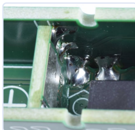
Figure 19. Don't forget to solder the positive supply rail connection from PCB2 to PCB6.
