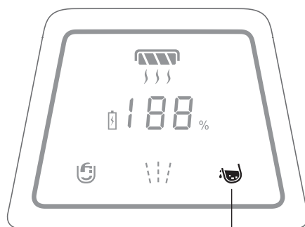
Clean water tank and filter
