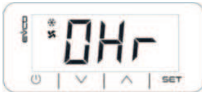
OHr Displays the hours of operation
