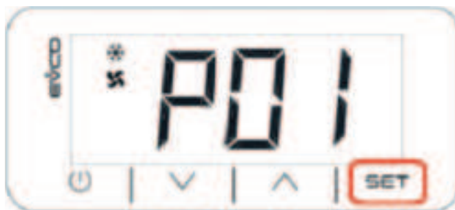
Step 6: Press SET , number displayed is minutes evaporator fan alternating on/off in non-cooling
