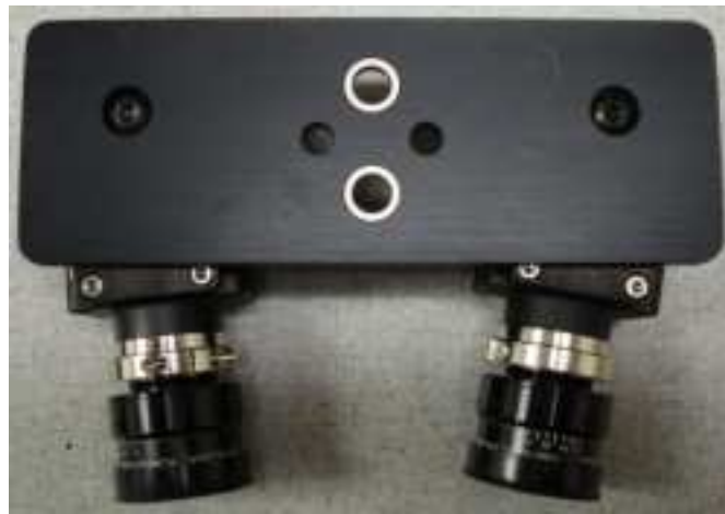
Figure 2.3 Camera Sub-assembly, Backside
