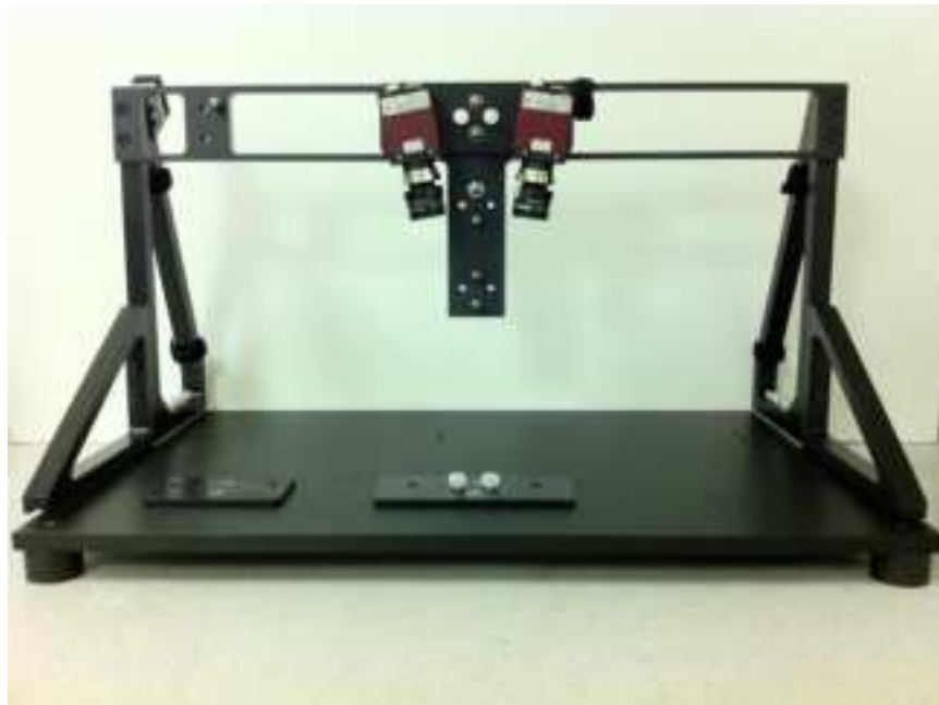
Figure 2.8 DIC System Installed on Standby Plate
