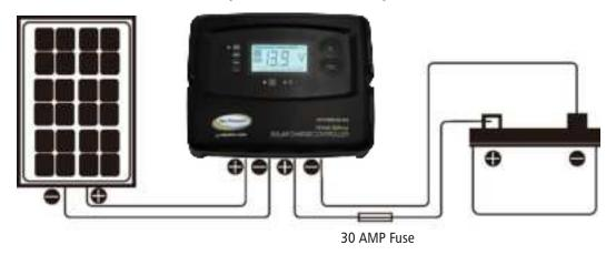
Note The fuse or breaker used should be no larger than 30 amps.
