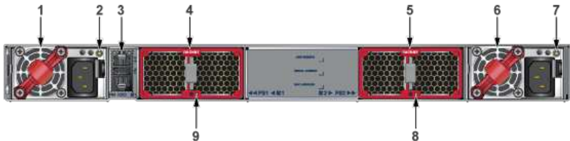
Figure 50: Rear Panel with Two Fan Modules (1RU)
