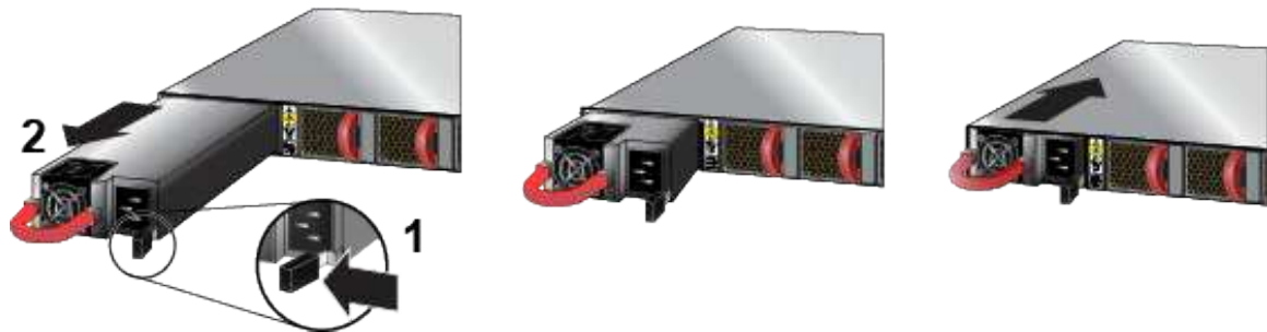
Figure 54: Removing and Installing Power Supply
