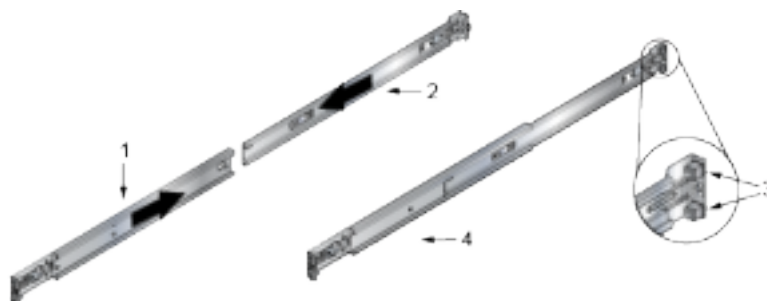
Figure 12: Assembling the Rails
