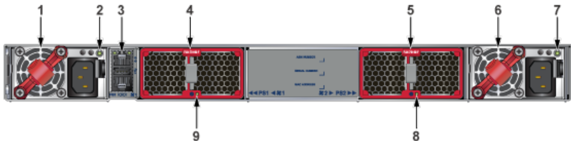
Figure 50: Rear Panel with Two Fan Modules (1RU)
